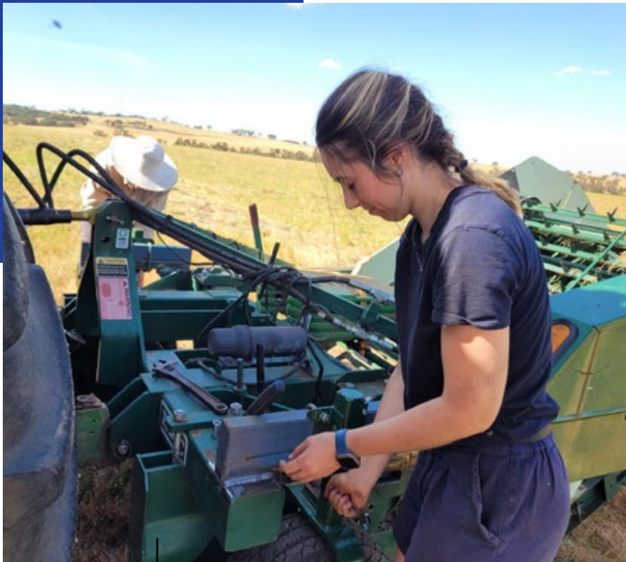
Ruby Wiese aiding in-field tuning of prototype machine for swathing subterranean clover during trial at UWA Farm Ridgefield in October 2023.
