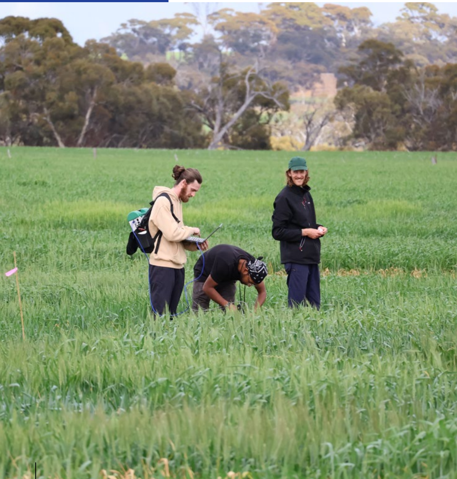
UWA students Ewen McCabe, Agyeya Pratap and Owie McCarthy collecting hyperspectral measurements of wheat flag leaves with the ASD FieldSpec 4. See page 105
