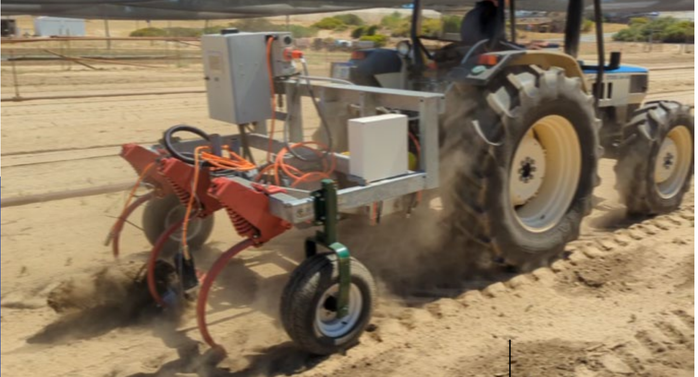
Testing of the prototype weed control device at the Shenton Park Field Station.
