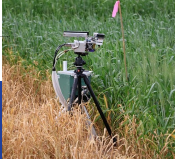
A LICOR-6400/XT portable photosynthesis system set up, ready to measure wheat flag leaf photosynthesis.
