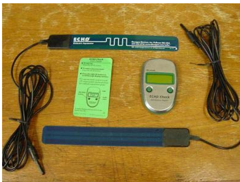
Figure 7: ECH 2 O soil moisture monitor (centre right) and two dielectric aquameters (top and bottom)
